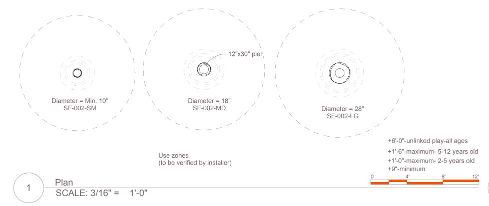
Installation Note: Max Fall Height above TPS: 2-5: 20" 5-12: 30" Installation Note: Finished height of stepping forms may be varied by lowering concrete footing. Installation is wet set. Safety surfacing (by others) Finished grade 1/2" Threaded insert 1/2x12" J Bolt 12" x 30" Fiber reinforced concrete pier by others Compacted subgrade (by others) Detail
